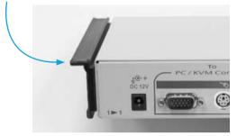
3. Fasten the console to the rack, using the provided screws.
